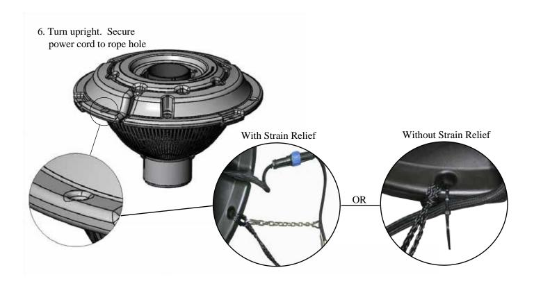
7. If ready to install in the pond, go to Installation instructions. Light Kits can also be installed at this time, go to Light kit instructions.
