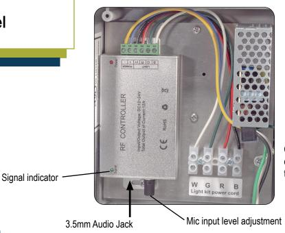
Connect light kit power cord wires to this terminal block.
