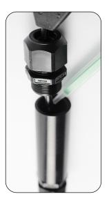
10. Hang the cord in a vertical position with the open end of the cable joiner (splitter side) on top. Use the potting kit to fill the inside of the cable joiner making sure the potting completely covers the black jacket of the splitter cord.
