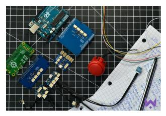
The Arduino Shield on the left allows you to add Wirelings to your Arduino projects. Featuring a 4-channel Multiplexer, Real-Time Clock (RTC), on-board voltage regulation and level shifting, this board allows you to add up to 4 Wireling sensors to your project with ease!
