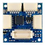
Moving up the electronic food chain we have the Wireling Adapter board (left) that connects all these external sensors to it by way of the supplied 5-pin connectors.
