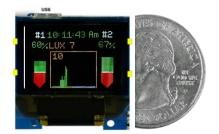
Arduino Zero) running at 48 MHz with 256K Flash, 32K RAM, a USB port, a real-time clock, power management, battery charger and, at the top, a 16-color 96h x 64v OLED screen all packaged into one square inch.
