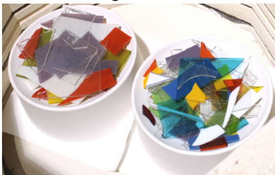
One Scrap Master filled with 44 ounces of COE90 glass and the other with 44 ounces of COE96 glass in a kiln ready to be fired.
