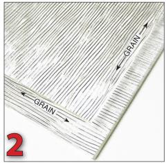
Lay the second Clear Cord square on top of the first, *textured side down*, turning the second square 90° so that the texture grains "crisscross." Full fuse using the basic System 96° 6-segment Firing Schedule on our website.
