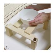
**Step 1:** Make sure that your kiln shelf is protected with kiln wash and level. Then, using a combination of kiln posts and Hot Damz, create a stand to elevate the Pot Melt mold of off the kiln floor. Make sure that the hole(s) in the mold are unobstructed and that the legs of the stand are far enough apart that the glass won't touch once it melts through.
