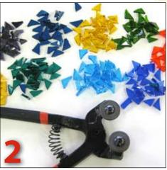
Using glass nippers, nip strips into small triangles.
