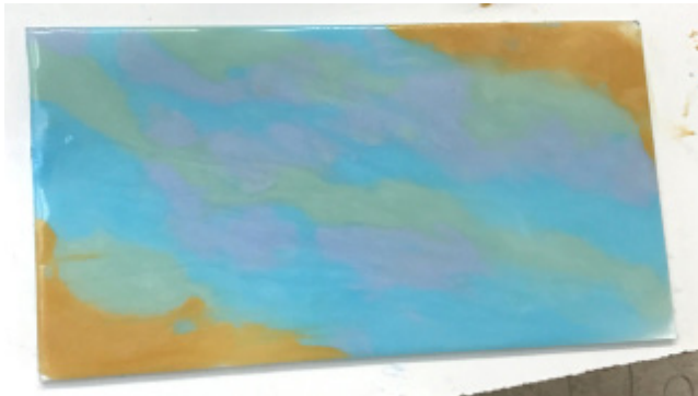
Image C. Spritz the slurries with water or gently vibrate the glass from side to side to create a smooth and even blend of frit colors.
