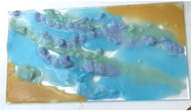
Image A. Place the frit slurries onto the glass.
