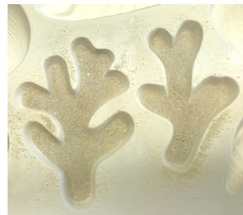
Add F2 Khaki until smaller cavity holds 19 grams and larger holds 25 grams total of frit.
