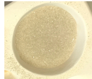
Add F2 Khaki until the cavity holds 20 grams of frit.
