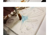
Begin by treating the mold with MR97/ZYP spray in a ventilated area. Several coats with a short waiting period between coats are preferable to one heavy coat. Be sure to hold the mold at various angles while spraying to assure that the spray gets to every vertical surface as well. Shake the can well before use and hold the can upright while using to assure proper distribution of product. Click here for a tutorial on applying the ZYP.
