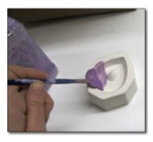
Apply the glass separator to the mold according to the manufacturer's instructions. Be sure to apply ample glass separator. If the glass separator is a water based product, it is crucial to drive the water out of the mold with heat/ evaporation before firing with glass.
