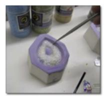
Fill the mold with another layer of medium grain clear frit (or other transparent frit color) The mold should be filled within 1/16" from the top of the frit cavity.
