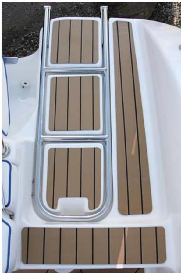
For larger area's follow the above guide. (Pictured below is the cockpit deck area of a Janmor 580. Note. the entire area was templated as one template made up from multiple pieces of paper)
