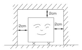
2. Make sure there is enough ventilation space around the sides and top of the refrigerator.
