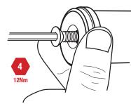
9 Pull the INNER clamp outward toward the SLI cap, ensuring there are no gaps between the grip sleeve and clamp. Torque clamp bolt to 15in/lbs. (1.7nm).
