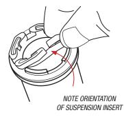
5 Install lock-on clamps and SLI end caps by aligning the grip sleeve (with suspension insert) with the pockets in the clamp and SLI end cap and press together.
