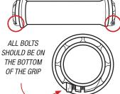
8 Position the clamp bolts downward (under the grip) and pull the inner clamp OUTWARD toward the bar end. Torque the OUTER clamp bolt to 15in lbs. (1.7nm).
