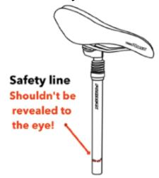
IMPORTANT! For safe and comfortable riding, there should be clearance of no less than 1-2 inches between the rider and the top tube of the bicycle frame, while the rider straddles the bicycle with both feet on the ground.
