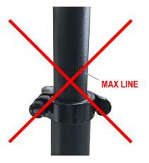
To do so, unlatch the quick-release lever on the seat tube and move the vertical stem to the appropriate height, making sure not to exceed the safety MAX mark. Point the front tip of the seat towards the handlebar along the frame. Close the quickrelease lever while making sure it's tight enough to keep the seat post in place.
