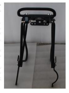
3. Put the rack arms on the frame and tighten the bolts slightly to the extent that rack arms can be moved by hand.
