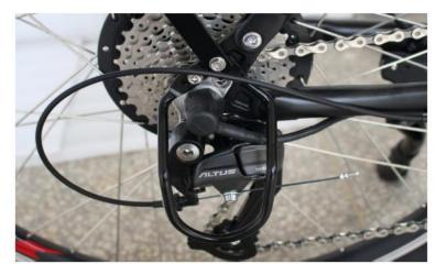
that it gets in the way of chain. The upper hole is for rack brace and derailleur guard on this side. Do not screw the bolts too tight for rack braces on both sides. It should be just tight enough to where the rack can be moved with a hand.
