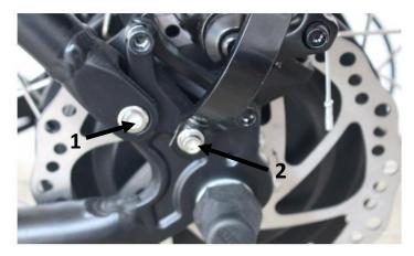
5. A Derailleur Guard will come in the parts box for you the bicycle. This should go between bike frame and rack brace on right side of the bike. The lower hole in the rear part of the frame is for derailleur guard AND rear fender brace support (if your bike has a fender). You will need to make sure the bolt for this hole is not too long
