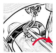
• Mount the fender's support pipes into the bottom of the fork (from both sides).
