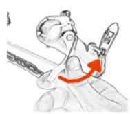
• Slide-in the handlebars bottom rod into the stem and lock the hoop back on it.
