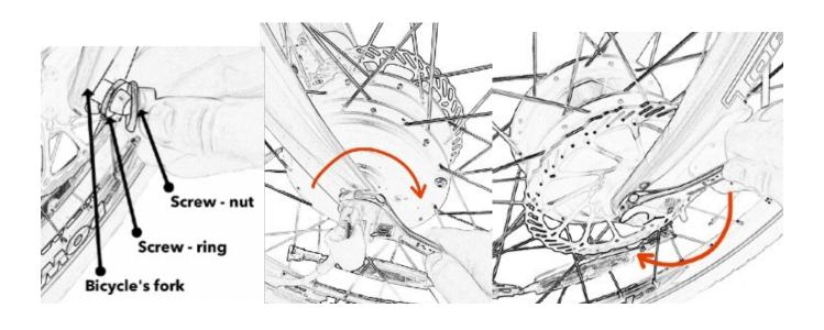
6. Connect the motor to its plug (arrow to arrow) and secure its wire with its screws to the fork.
