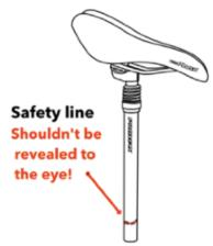
The height of handlebar's stem must be adjusted to the height of the user. The desired height is the most comfortable height to the user. <a href="Important!">Important!</a> – To avoid component breakage, when raising the stem, make sure that its safety line is unrevealed
