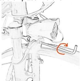
5. Assemble the front wheel and front fender to their place in the fork.
