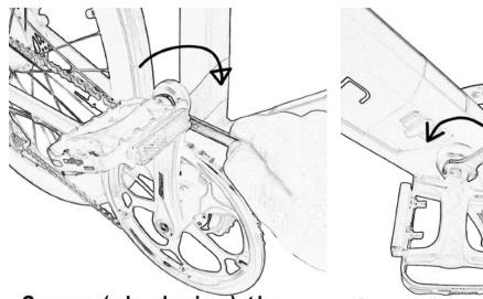
Screw (clockwise) the right pedal into its place
