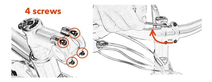
2. Adjust the handlebar so that it is aligned with the bicycle's fork. (2 screws).
