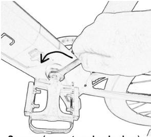
Screw (counterclockwise) the left pedal into its place
