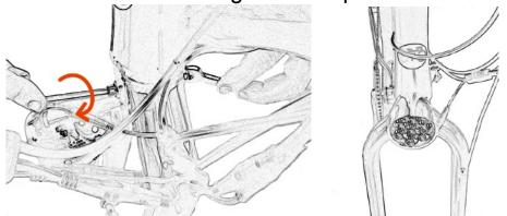
5. Assemble the front wheel by sliding the "wheel lock pin" through the bicycle's fork intended holes and into its place in the wheel, screw the screw-nut to the pin and lock it.
