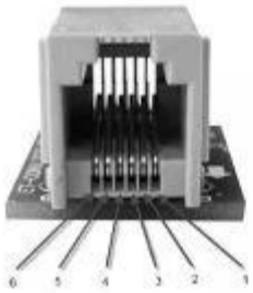
Hayward GLX-PCB-XXXX RJ11 Conn Jack Pinout
