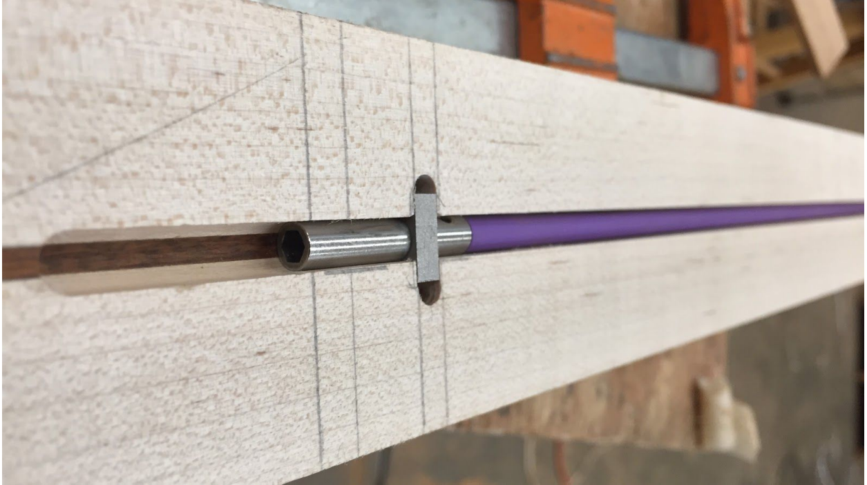
36. Here is a photo of the completed routing with a good view of the round-bottomed channel.
