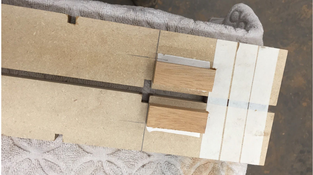
14. Here are the spacers attached to the bottom of the jig at the peghead end with double-sided tape. These spacers were milled to a thickness of .482" minus the thickness of the double-sided tape.
