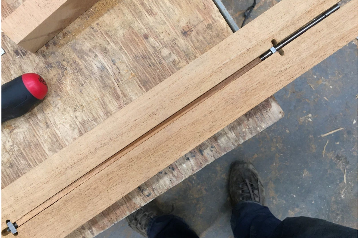
48. This photo shows the trussrod placed in the neck blank. For this build, I must bring the neck much further to completion before permanently installing the rod.
