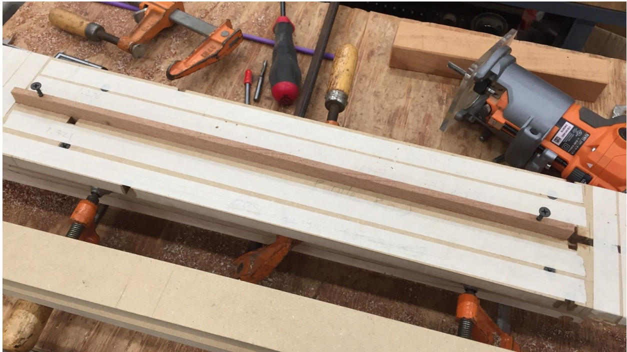
48. This photo shows the trussrod placed in the neck blank. For this build, I must bring the neck much further to completion before permanently installing the rod.
