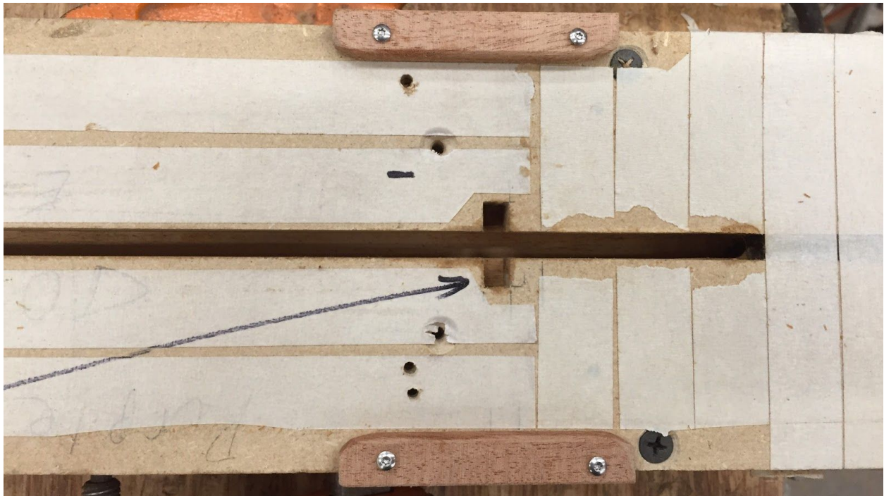
45. I didn't want the channel routing to interfere with the notches, so I screwed on these router base guides to keep the bit from meandering into the notches. Looking closely, you can see that they did their job.
