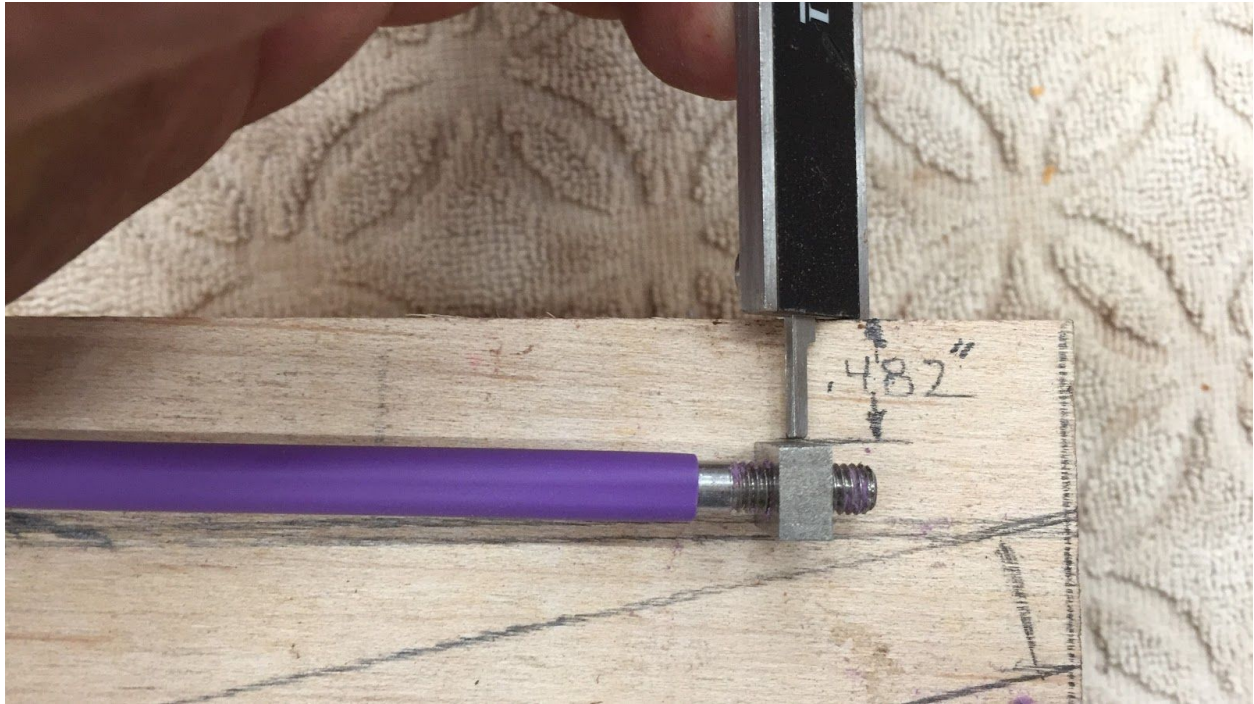
13. With the rod laid in place on the neck blank along its intended line of depth, I measured the space between the top of the endblock at the heel end of the neck and the top of the neck blank, or neck/fretboard interface. This is the exact thickness of the spacers we are going to add to the underside of the jig where the endblock notches are on the peghead end (in most cases the adjustment end) of the jig.
