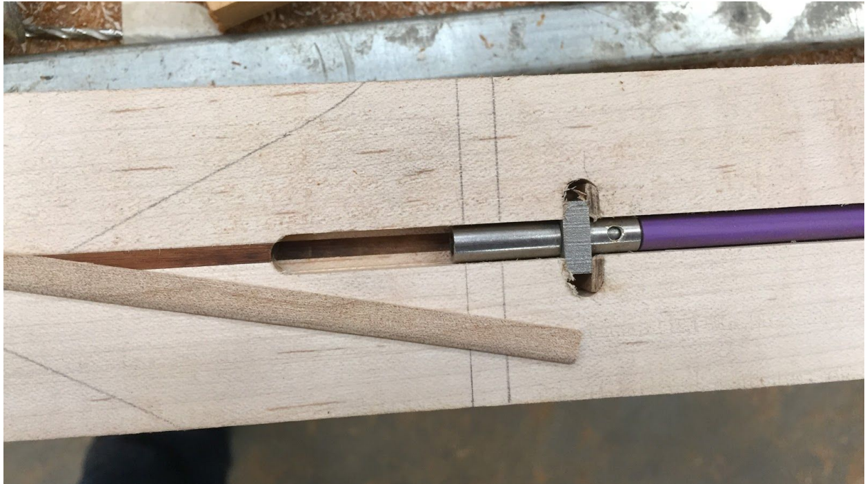
26 a, b. Once the rod is in place, turn the adjustment nut counter-clockwise until the outsides of the endblocks are firmly buttressed against the walls of the notches, as shown.
