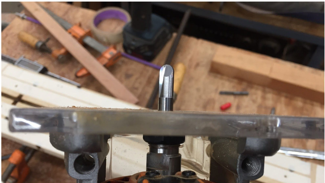
30. The steps for the second version of routing the cavity are much the same as the first, but with a few different steps. Here, you can see the cutter that will be used for the main channel,
