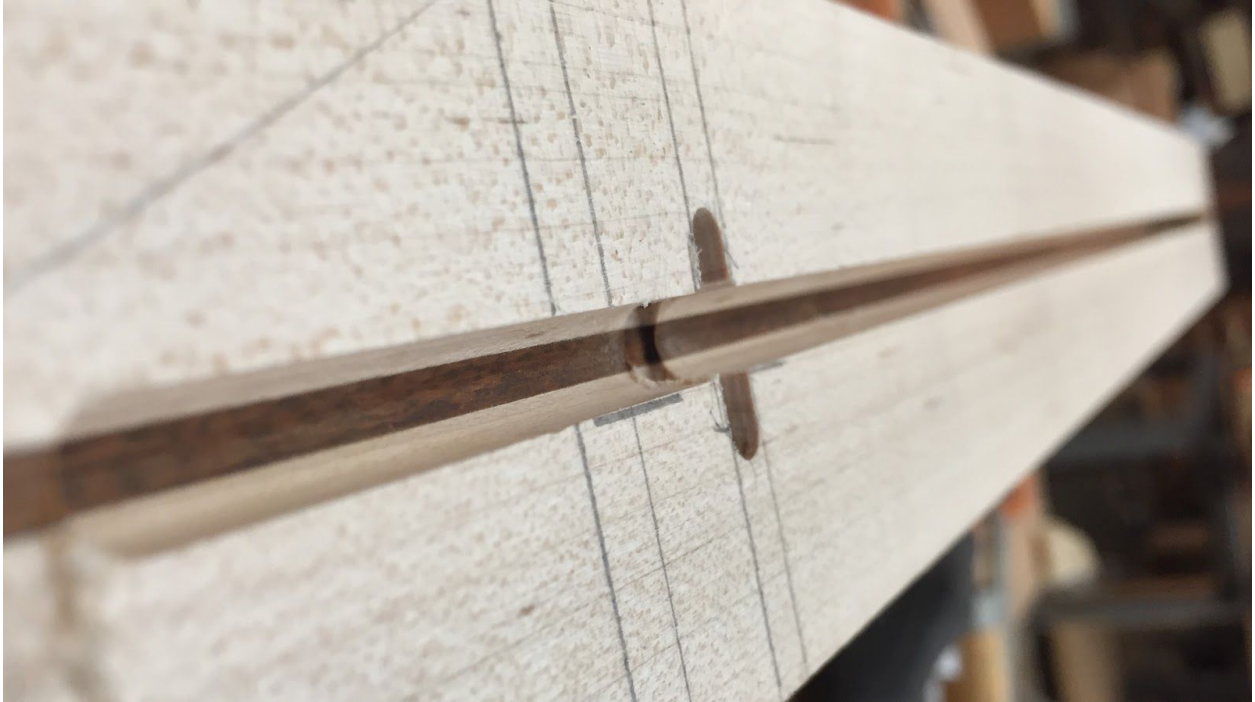
36. Here is a photo of the completed routing with a good view of the round-bottomed channel.
