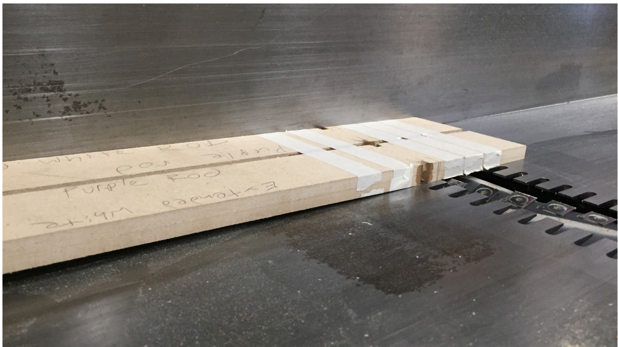
15. Once the spacers are in place, MDF must be removed from the bottom of the jig at the opposing end such that the far edges of the endblock notches meet the top surface of the neck blank. An easy way to do this is to pass the heel end of the jig repeatedly over a jointer blade until the proper amount of material is removed, as shown in the next photo.
