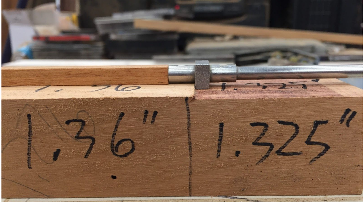
44. This is a photo of the rod sitting atop the router bit height block I made for this neck rout.
