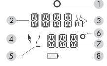
On the EL Range, the target mark and display are in the right optical channel. The brightness of the display can be set to one of five levels using the LIGHT menu option. The binoculars automatically adjust the selected brightness of the display based on ambient light levels.
