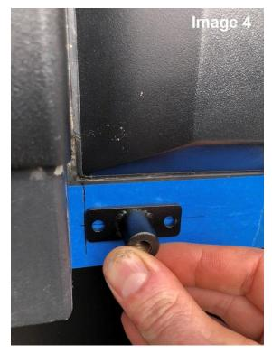
**Step 5:** Using the lower strut mount, align the outside edge of the mount with the vertical line you drew in Step 4. Center the mount vertically on the horizontal line; see Image 4. Mark the hole locations on the tape and remove the lower mount. Repeat this step on all 4 taped locations. Do not drill as this time. Continue with Step 6, as we will verify the lower mount location.
