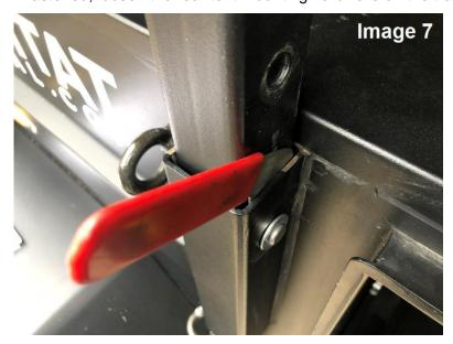
wood, sheet metal or small screwdriver into the front rack mounting tube in order to center the front tube within the larger mounting square; see Image 7. Now adjust the rear mounting rack against the tent mount to center the rack within the larger mounting tube. Once close, tighten down the tent mounts and verify the position. Be patient and work from side to side, this step is important.
