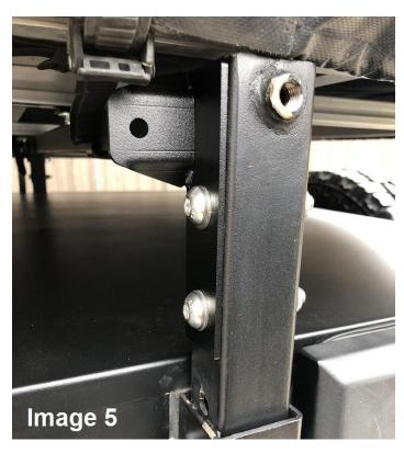
Step 7: After verifying the measurement, center punch the mounting location of the two holes for the lower strut mount. Drill lower mount holes; we recommend starting with an 1/8" pilot drill bit and finishing with the 1/4" drill bit. Repeat on all 4 mounting locations and deburr holes.
