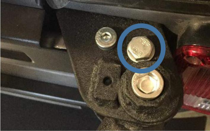
Repeat the process for the lower door hinge. (note: Lower body hinge bracket does not have an elongated hole.)
