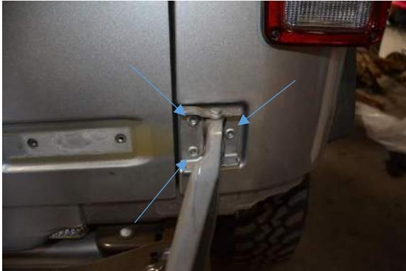
Step 4: On the bottom of the hinge grind the hinge pin smooth with the hinge using a grinder.
