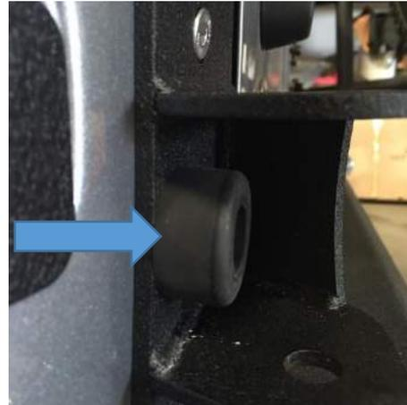
Step 21: Install the rubber bumper stops to the last two mounting holes with the provided hardware using the two button head bolts and secure with nuts. (note: Do not over tighten or you will collapse the stopper.) The rear body mounting plate is now fully installed. Reinstall brake light housing and don't forget to plug the rear light harness back into the housing.
