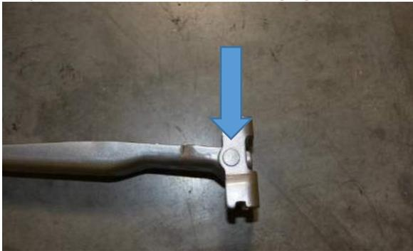
Step 5: Using a punch, drive the factory hinge pin out with the hinge supported in a bench top vise.
