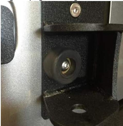
Step 22: Tire carrier adjustment up or down to ensure proper alignment with rear body plate. The upper body hinge has an adjustable cam, turn clockwise or counter-clockwise to move tire carrier up or down. Once you have centered the tire carrier so that it engages smoothly with the body plate secure hinge bolts and tighten.
