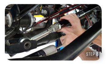
STEP 9: If the bolt gives you a little trouble as it does not line up perfectly. Tighten the strap a little more if possible so the bolt easily goes through.
