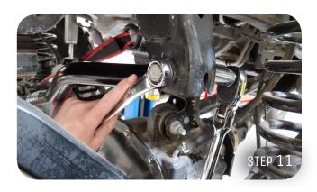
STEP 12: Next using the large crescent wrench tighten the 2 adjustment nuts
