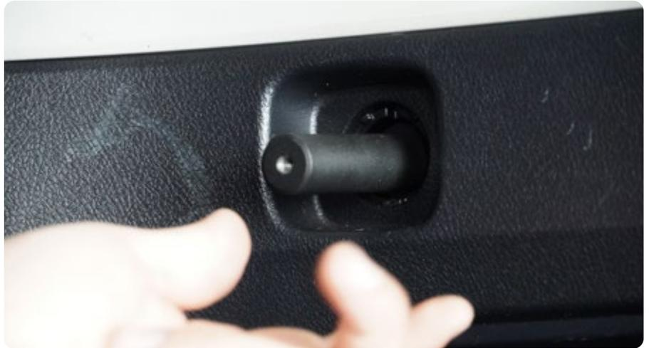
**STEP 7** | Begin installing molle panel by securing it to the factory mounting location above the rear window using the factory bolt and a 10mm socket.
