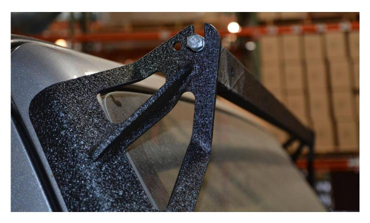
7) Rotate the center mounting bar to line up to the second threaded hole with the hole located on the A pillar mounting bracket. Install the second bolt to lock the center bar in place.
