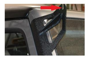
5) Locate the front threaded hole on the center section of the LED light bar (shown below) and place the 13mm bolt with a washer and a lock washer partially threaded into the hole (shown below)
