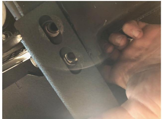
17) Hold the bumper up to where the OEM bumper was mounted. The two frame rail brackets will slide over the frame as shown in the illustration below.
