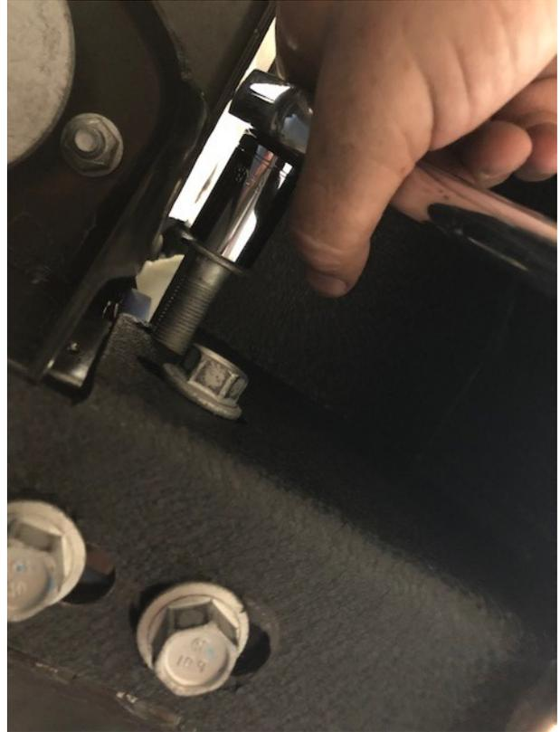
19) Use the two large kit bolts on the passenger side where the nut plate was installed in step 16. Tighten to 80 ft/lbs.
