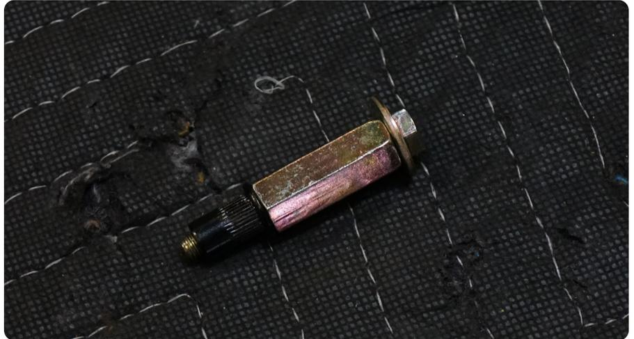
**STEP 17** | Slide the nutsert tool with the nutsert into the mounting hole. Ensure the flange of the nutsert is flat against the vehicle prior to tightening.
