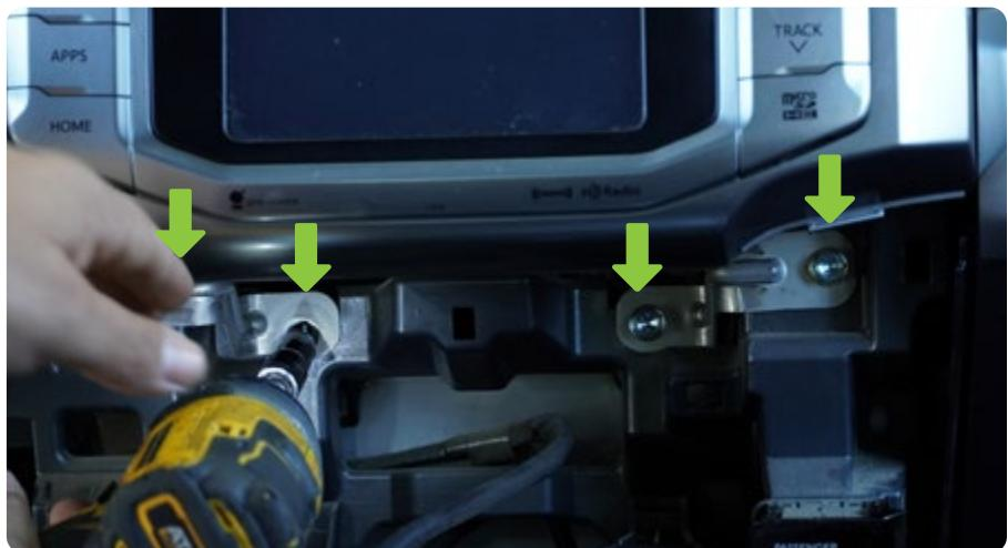
**STEP 5 |** Drill out the marked holes using an 11/32" drill bit.
