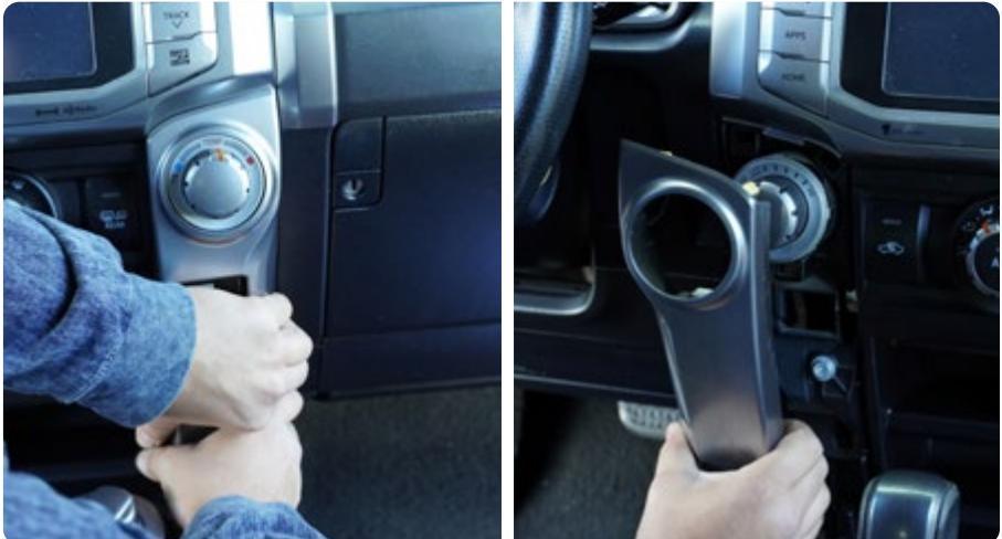
**STEP 2** | Remove the control cluster by pulling towards the rear of the vehicle to release the clips, and disconnect the wiring connector on the back.
