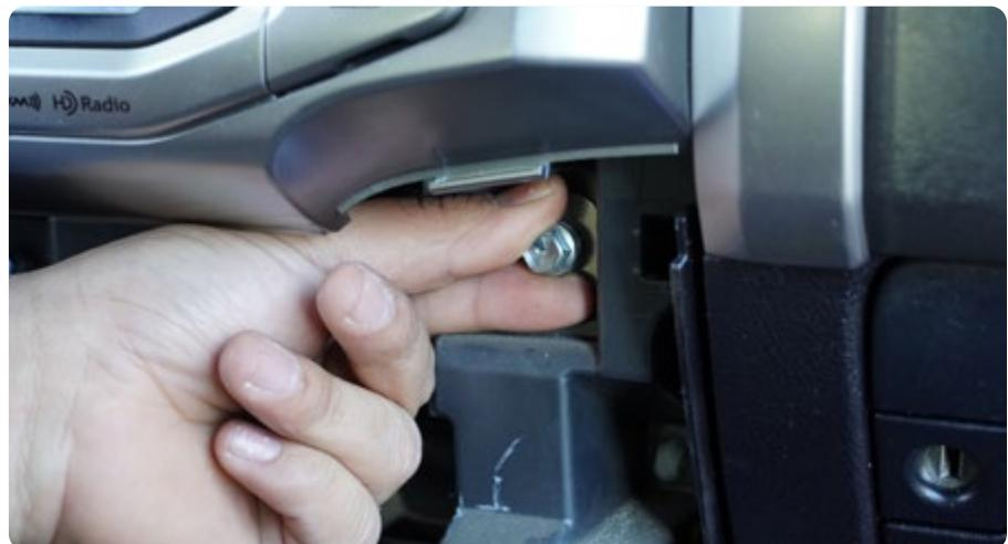
**STEP 8 |** Install the control cluster and dash trim by applying pressure until the clips are secured.
