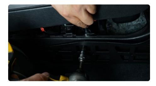
STEP 6 Once panels are installed, push center back down into place and ensure clips are secure. Reinstall shifter knob and boot.
