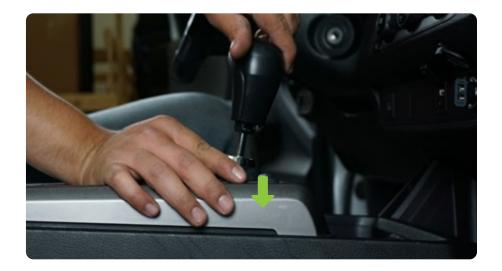
STEP 4 | Gripping the top of the center console, pull up to release the clips until the center console is free.
