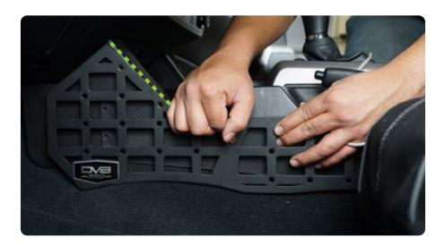
STEP 2 | Once all holes are marked, using a 11/32" drill bit, drill the holes only cutting through the plastic of the center console.
