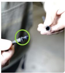
STEP 24 | Connect the camera wiring harness by pressing it into place until the clip is secure.
