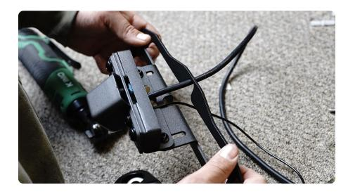
STEP 19 | Align the upper bracket so that it is straight and even, then secure the M6 hardware using a 4mm allen bit.
