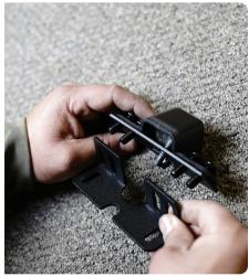
STEP 14 | Place the mount cover over it, and loosely secure with the provided M8 hardware.
