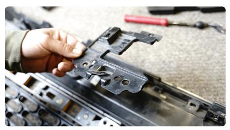
STEP 12 | You can now remove the camera housing assembly.
