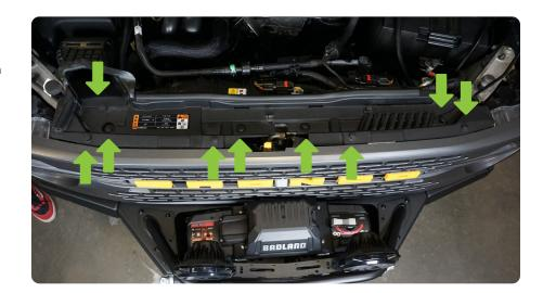
STEP 2 | Move the air intake cowl up/ back and out of the way.
