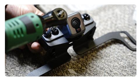
STEP 17 | Install the included extended camera wire to the camera.
