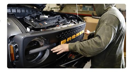
STEP 26 | Use a 13mm socket and the factory hardware to secure the grille to the vehicle.
