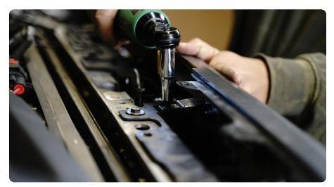
STEP 27 | Place the plastic grille trim back into place above the grille and pull the factory air intake cowl. Secure using the factory plastic grille trim using the factory push clips.
