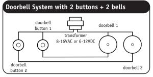
Bell 1 rings when button 1 is pushed and Bell 2 rings when button 2 is pushed.
