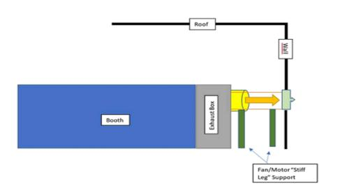
Additionally, most municipal codes require that ductwork be at least 6 above the ceiling exit point as shown above. This requirement will also apply to wall-exhausted systems as well unless otherwise approved.
