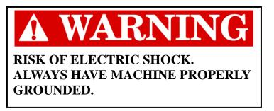
Your mixer **MUST BE PROPERLY GROUNDED**. If there is an electrical short circuit, grounding reduces the risk of electric shock.
