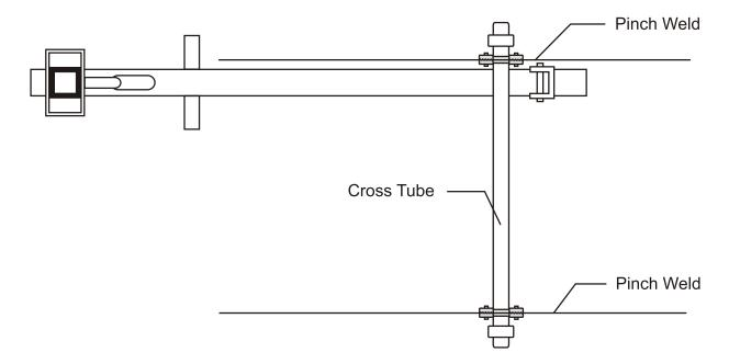
For pulling one side only, it is best to attach the cross tube to both rocker panels. Anchor your body straightener to the cross tube. This will prevent unwanted rolling of the underbody clamps on the pinch weld.
