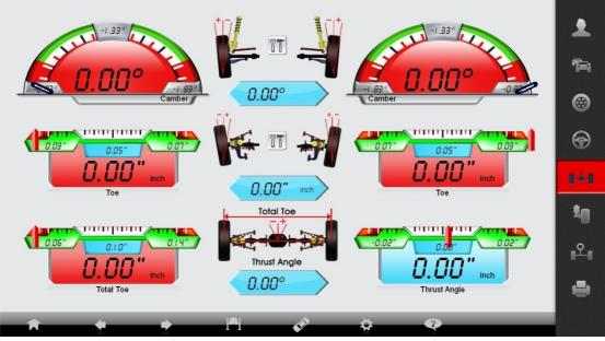
Diagram: Standard Measurement – Rear Axle
