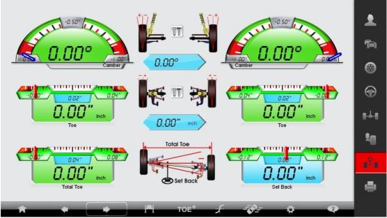
Diagram: Standard Measurement - Front Axle
