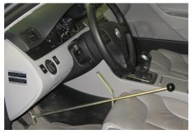
Place a cloth underneath the depressor to protect the seat if necessary. After run out compensation, install the brake depressor for further measurements.
