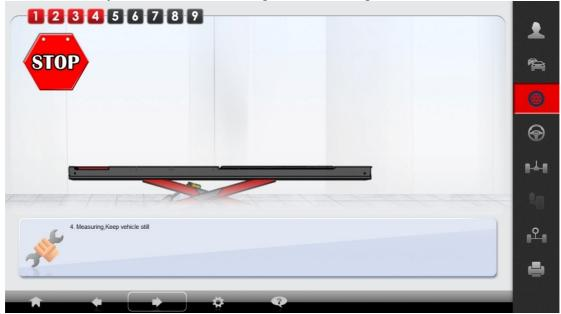
Diagram: Standard Measurement: Run Out Compensation
