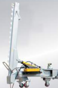
10 Ton Pull Tower w/ Multi-Angle 360 degree Pulling Capability
