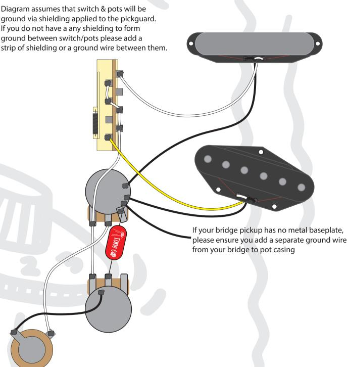
This diagram has been drawn with traditional 2 conductor pickup wires in mind. If your pickup is different to this, then please refer to that manufacturer's wire colour coding prior to installing.
