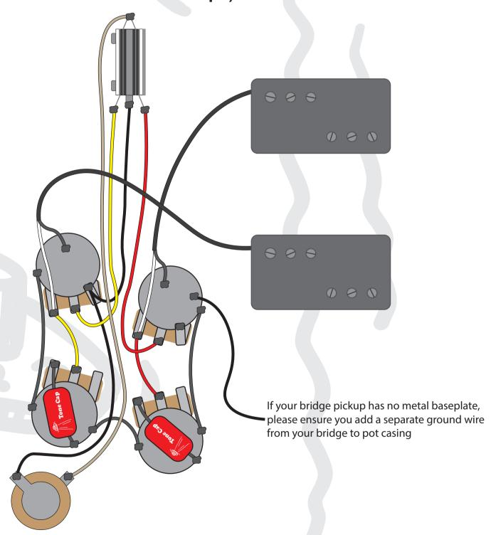
This diagram has been drawn with traditional 2 conductor pickup wires in mind. If your pickup is different to this, then please refer to that manufacturer's wire colour coding prior to installing.
