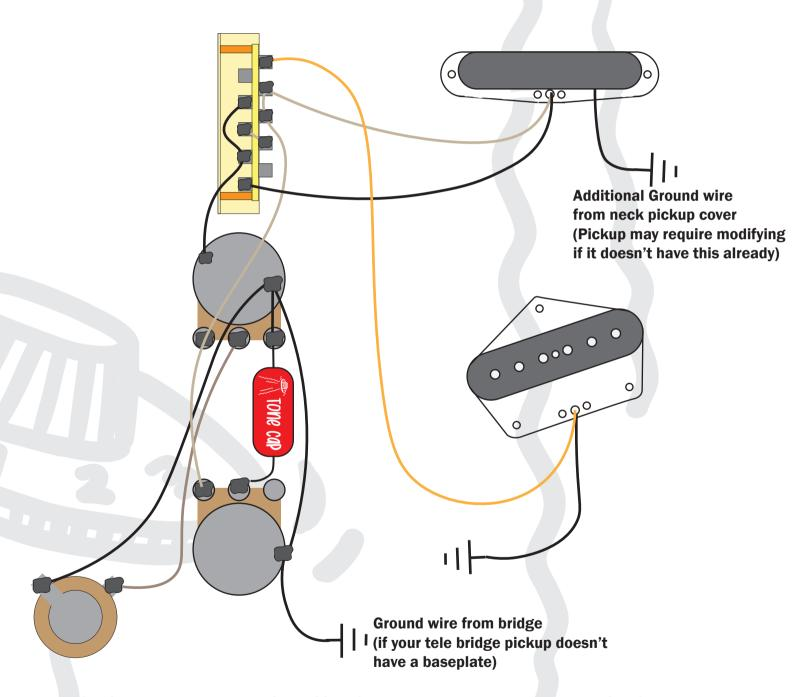
Our diagrams have been drawn with traditional 2 conductor cloth covered and/or outer braided 2 conductor pickup wires in mind unless otherwise stated. Your pickups may have a different wiring style, so consult with your pickup manufacturer for the correct wire type and/or colour coding before installing.
