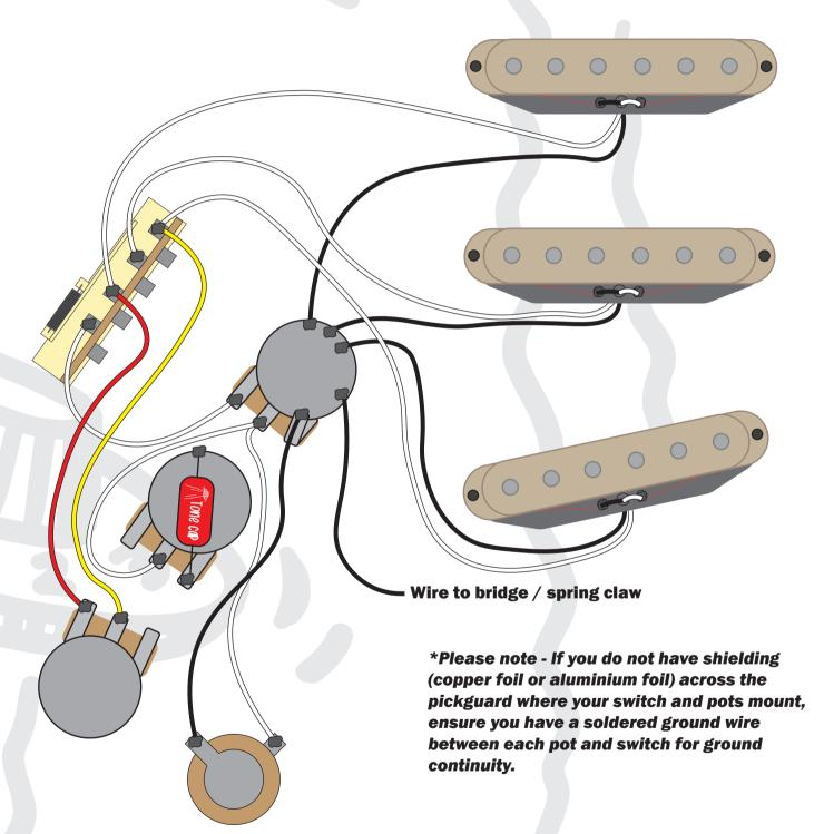
This diagram has been drawn with traditional 2 conductor braided pickup wires in mind. If your pickup is different to this, then please refer to that manufacturer's wire colour coding prior to installing.
