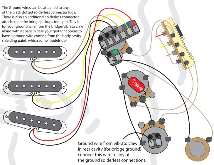
Our diagrams have been drawn with traditional 2 conductor cloth covered and/or outer braided 2 conductor pickup wires in mind unless otherwise stated. Your pickups may have a different wiring style, so consult with your pickup manufacturer for the correct wire type and/or colour coding before installing.
