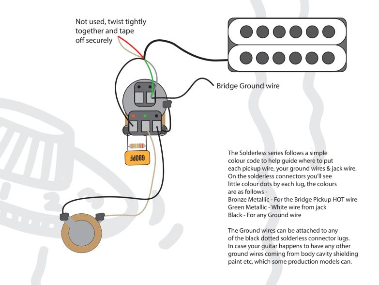
This diagram has been drawn with the Seymour Duncan Invader pickup wire colour codes in mind. If your pickup is different to this, or importantly, a different pickup manufacturer, then please refer to that manufacturer's wire colour coding prior to installing.
