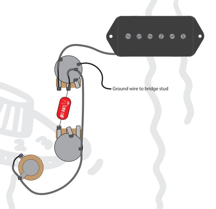
This diagram has been drawn with traditional 2 conductor braided pickup wires in mind. If your pickup is different to this, then please refer to that manufacturer's wire colour coding prior to installing.
