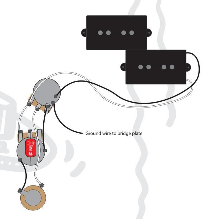
This diagram has been drawn with traditional 2 conductor braided pickup wires in mind. If your pickup is different to this, then please refer to that manufacturer's wire colour coding prior to installing.
