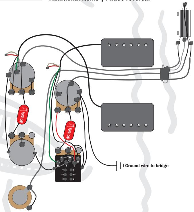
This diagram has been drawn with Seymour Duncan wiring colour codes in mind, where black is the hot, green and bare are ground and red & white are for series link. Your pickups or pickup brand may use different colour codes, please ensure that you have confirmed your pickup and manufacturer's own colour before commencing with install.
