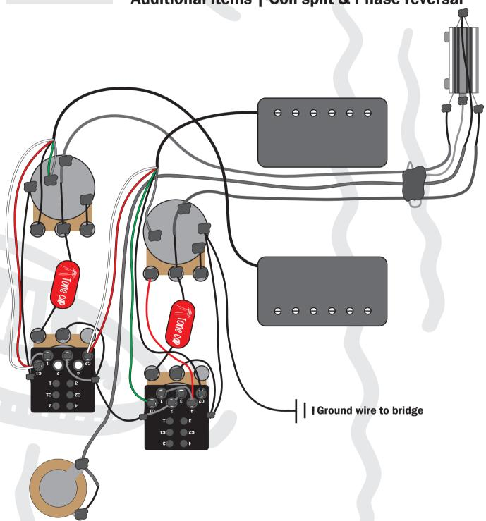
This diagram has been drawn with Seymour Duncan wiring colour codes in mind, where black is the hot, green and bare are ground and red & white are for series link. Your pickups or pickup brand may use different colour codes, please ensure that you have confirmed your pickup and manufacturer's own colour before commencing with install.
